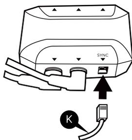
With both bases in FLAT position, connect each base to the other by inserting each control box slot labeled sync. NOTE: If using 3-in-1 legs, BOTH bases need to be converted to the 3-in-1 to maintain consistent deck height
