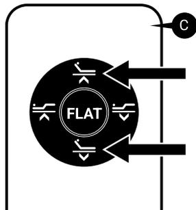
Simultaneously press and hold the HEAD UP and HEAD DOWN buttons on remote until the remote back lights blink, then release remote buttons.
